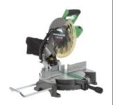
Feat. Hitachi's Laser Marker for increased cutting accuracy; 15 Amp motor; 0-52 Degree miter angle range to right & left; 0-45 Degree bevel angle range to left; Horizontal handle; Large pivoting flip fence raises 4"; Large table; Thumb actuated positive stops; Carbon brush access; Dust collector minimizes airborne particles; Weighs 26.5lbs. Includes Saw Blade; Pivoting Flip Fence; Dust Bag; Vise Assembly; 10mm Box Wrench & 4mm Hex Bar Wrench.
