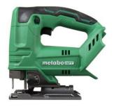
This jigsaw is capable of generating a no-load speed of 2,500 SPM for a variety of wood and metal cutting applications. It features and LED light; dust blower; 3 orbital functions plus a standard straight-cut mode allow for faster cuts; 45 degree left and right adjustable base; tool-less blade change; quick brake function; battery charge indicator; variable speed trigger for ultimate control and ergonomic D-shaped handle with elastomer grip. Weighs 4.2 lbs. Lithium Ion Lifetime Tool Warranty.
