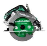
Circular saw features Torque Boost Technology which automatically switches the saw from high speed to high torque for tougher cuts or thicker wood. It has an industry leading speed of 6,000 RPM and the new visible cutting depth indicator ensures a precise cut every time. It has a 2-7/16" cutting depth with a 55 degree bevel capacity for deep and accurate cuts. Accepts any MultiVolt battery and can also accept the unique AC Adapter to plug in for all day runtime. Lifetime tool warranty.
