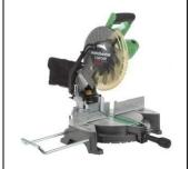
Feat. Hitachi's Laser Marker for increased cutting accuracy; 15 Amp motor; 0-52 Degree miter angle range to right & left; 0-45 Degree bevel angle range to left; Horizontal handle; Large pivoting flip fence raises 4"; Large table; Thumb actuated positive stops; Carbon brush access; Dust collector minimizes airborne particles; Weighs 26.5lbs. Includes Saw Blade; Pivoting Flip Fence; Dust Bag; Vise Assembly; 10mm Box Wrench & 4mm Hex Bar Wrench.
