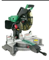
The C12FDH 12" Dual Compound Miter Saw features Hitachi's laser marker system for cutting accuracy. The saw head bevels to the right or left- allowing the material to stay securely in place for ultimate cutting efficiency. It cuts various types of wood, crown molding, plywood, decorative panels, soft fiberboard, hardboard and aluminum sashes.
