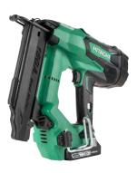
The NT1850DE 18-Gauge Cordless Brad Nailer allows the user to move easily around the jobsite without hoses or compressors! Equipped with Brushless motor technology and powered by a Compact 3.0Ah Lithium Ion battery, it is capable of driving up to 1,650 nails per charge. It employs a unique air spring drive system (similar to Hitachi's pneumatic line) that uses compressed air to drive each nail resulting in zero ramp up time.
